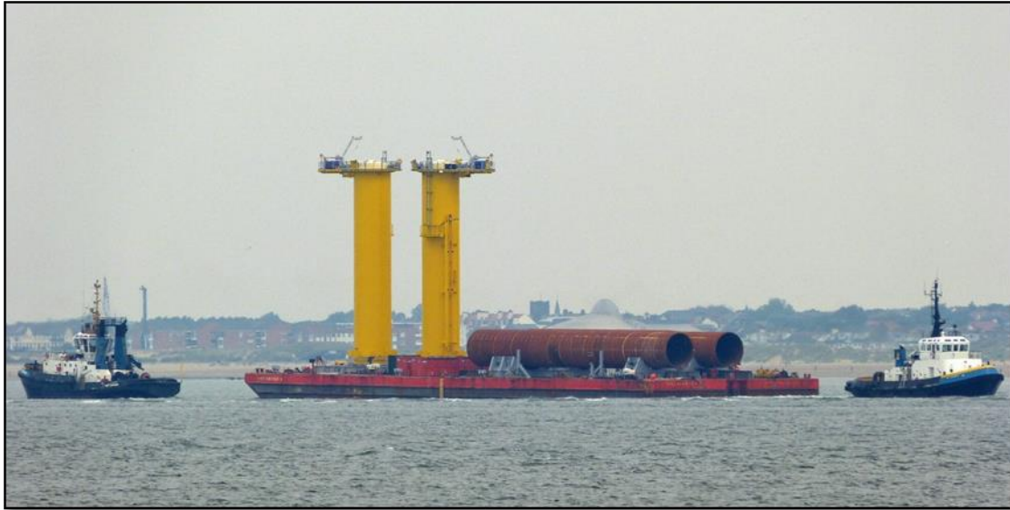
Figure 2-14. Monopile foundations and transition piece. Source: ARG-Flickr (2012).
