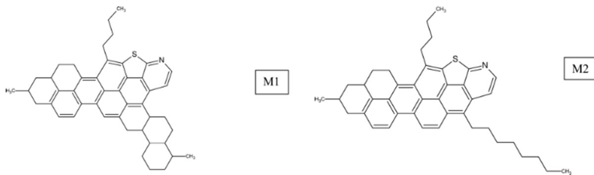
Figure 3.7. Representation of chemical structures for the fractions A1 (M1) and A2 (M2) of asphaltenes. Original figure from (ACEVEDO, 2018), reprinted with permission. Copyright (2020) American Chemical Society.
