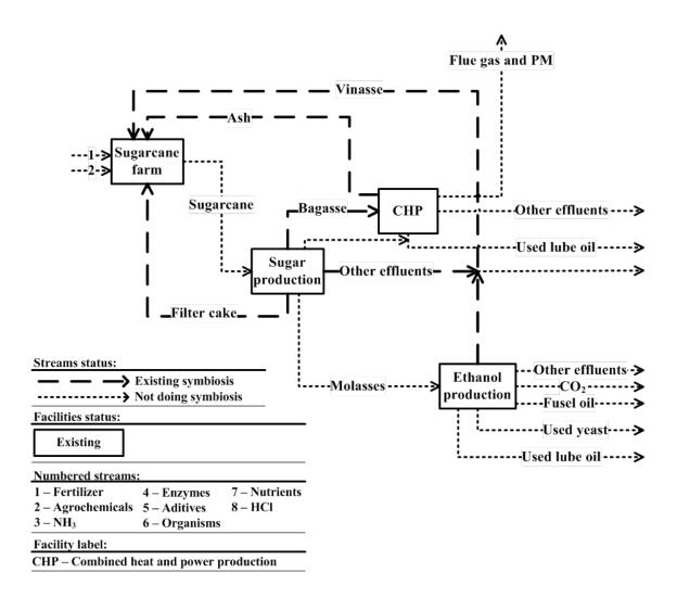
Figure 5.7: Diagram of the reference configuration. Source: Prepared by the author.
