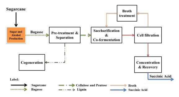
**Figure 5.2:** Simplified diagram of the Fermentation to Succinic Acid production. Source: Prepared by the author from [244].
